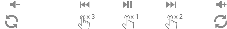
Counterclockwise rotation (Reduce volume) Press three times (Previous Song) Press Once (Pause) Press twice (Next Song) Clockwise rotation (increase volume)
